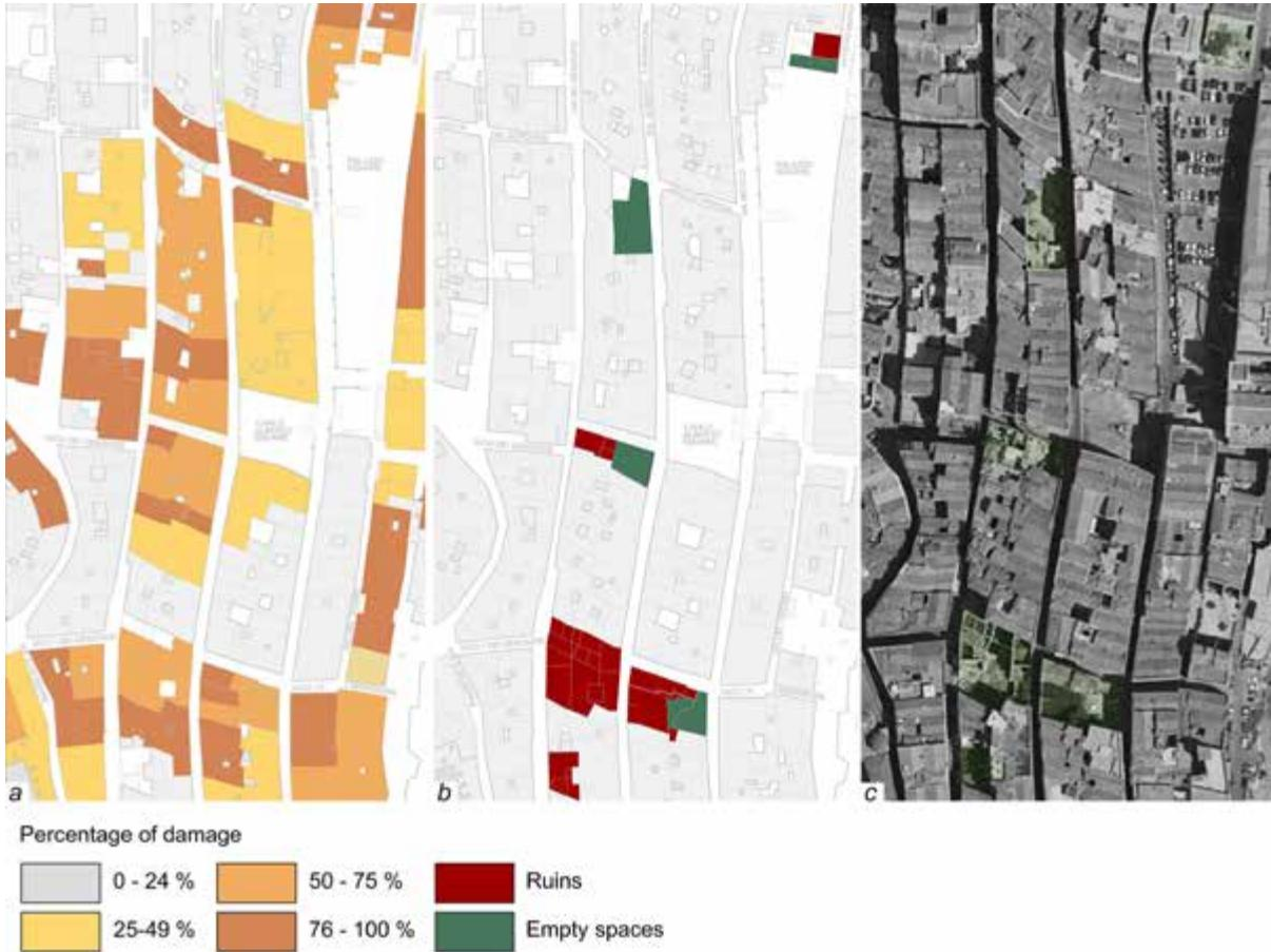
Figure 12. Particular portion of Castello quarter a) re-elaboration of the Genio Civile post-war cartography with the percentage of damage; b) current survey showing the presence of ruins and empty spaces from bombings; c) orthophoto with highlighted the neglected areas (elaboration by E. Pilia).
