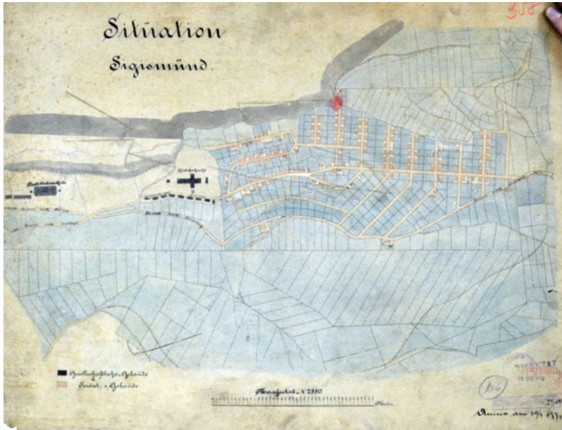
Figure 5. Sigismund Colony planned to be developed in connection with one of the mine's exploitation shafts, dated 1877: (black) the exploitation site, (pink) miners' dwellings, (blue) property lots. Anina Mine Archive, 1877.
